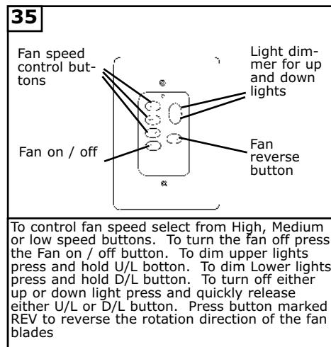
35 To control fan speed select from High, Medium or low speed buttons. To turn the fan off press the Fan on / off button. To dim upper lights press and hold U/L button. To dim Lower lights press and hold D/L button. To turn off either up or down light press and quickly release either U/L or D/L button. Press button marked REV to reverse the rotation direction of the fan blades
